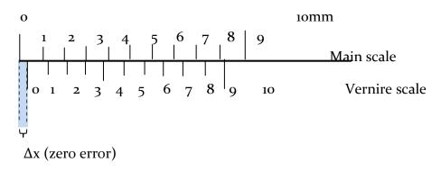
Zero error of the instrument = 0.3 mm.
