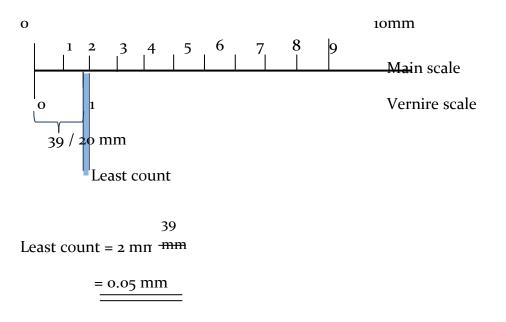
A sliding vernier caliper is shown in the figure above. Its shaded part is called 'fixed jaw'. Main scale is marked on the fixed jaw. And vernire scale is marked on the sliding jaw scale. Lock nut is used to keep the sliding jaw stationary. When the jaws are closed together, zero of the vernire scale and zero of the main scale coincide with each other. Then the jaws will exist in position as follows.
